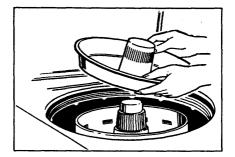
5. After loading clothes into the Mini-Basket tub, be sure to replace the Filter-Flo pan. The pan serves as a lid to keep the clothes in the Mini-Basket tub.
